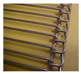
Lumsden's <u>Edgewise</u> edge has proven to many customers that this design prevents tangling and catching of the wires both on and off the machine. They come off the rolls untangled, they don't catch on adjoining belts, and there are no ends to bend open and break.
