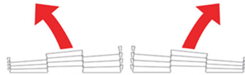
Lumsden Turn Belts are available in 90 and 180 degree turns, in all the standard sizes. Made of 302 Stainless Steel, it will run perfectly on your current turn conveyor using the same sprockets.
