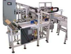
into the case packer. Intermittent or continuous flow of product and cases are controlled by servo motors. Horizontal and vertical case packers are available to meet your specific requirements.
